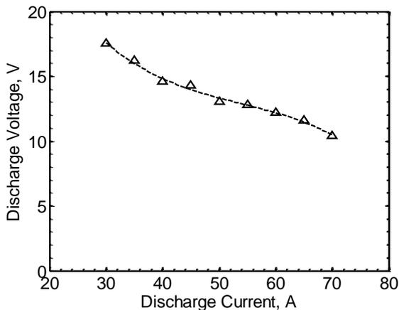
Figure 5. Theoretical electrical characteristic of the HC60 (5 mg/s Xe).
