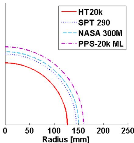
Figure 2. Outer channel radius comparison of various 20 kW-class Hall effect thrusters
