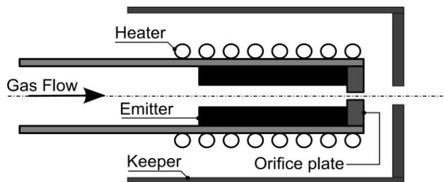
Figure 3. General schematic of an orificed hollow cathode.
